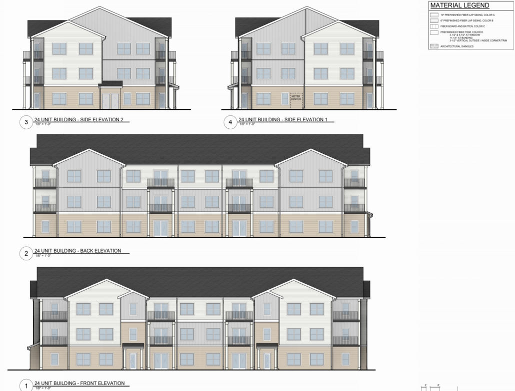
24-unit building elevations, sheet A-200 (Rosemann & Associates)
